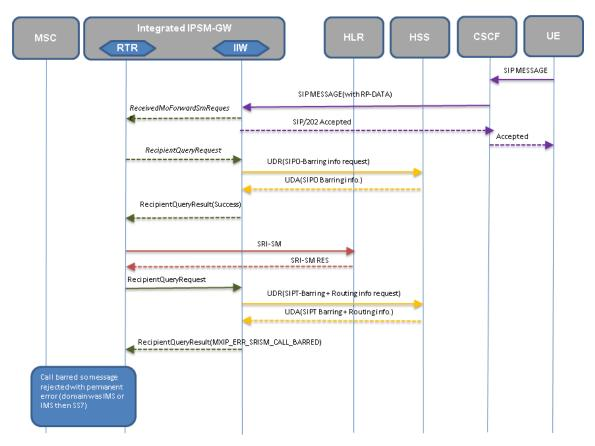
Figure 61: SIPO-SIPT scenarios where SIPO is not barred and SIPT is barred
