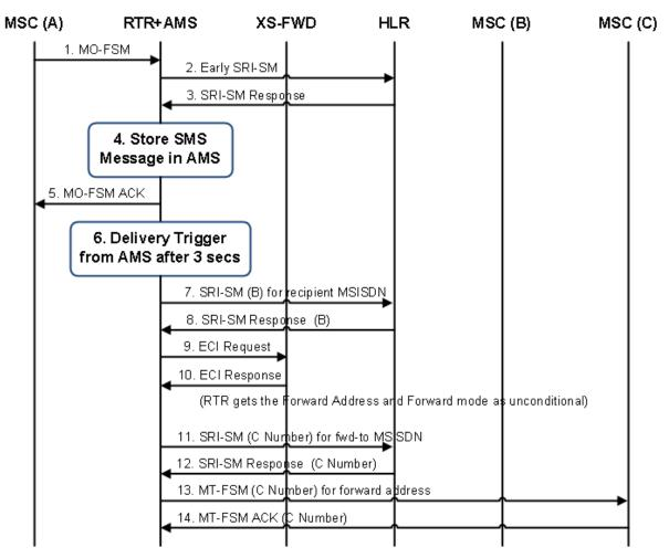
Figure 13: MO-Store-MT Scenario for unconditional XS-FWD service when rtrskipsrismforunconditional forwarding is false
