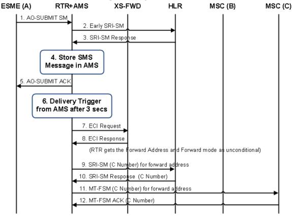
Figure 17: AO-Store-MT Scenario for unconditional XS-FWD service when rtrskipsrismforunconditional forwarding is true
