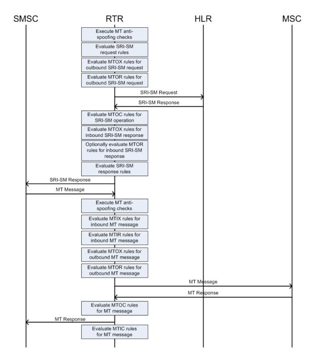
Figure 39: MT-MT routing example
