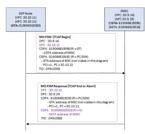
Figure 35: MO-FSM closed using TCAP-End or Abort
