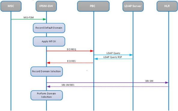
Figure 54: Mobile Domain via PBC and LDAP Server
