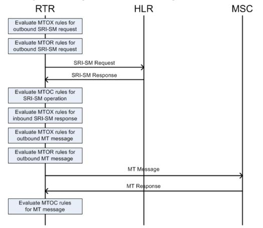
Figure 38: MO-MT routing example
