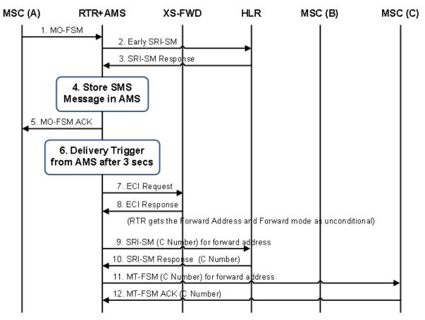
Figure 14: MO-Store-MT Scenario for unconditional XS-FWD service when 'rtrskipsrismforunconditionalforwarding' is true
