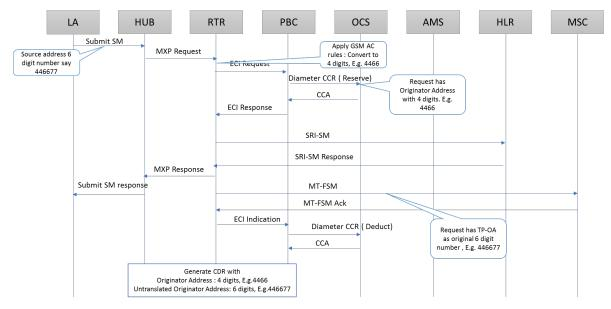
Figure 21: Flow Diagram where a Diameter server is used for charging
