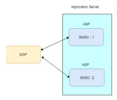
Sample M3UA SGP configuration for above application server:
