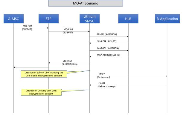
Figure 83: Flow Diagram for MO-AT Scenario
