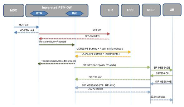
Figure 60: MO-SIPT message flow when the SIPT message does NOT get barred
