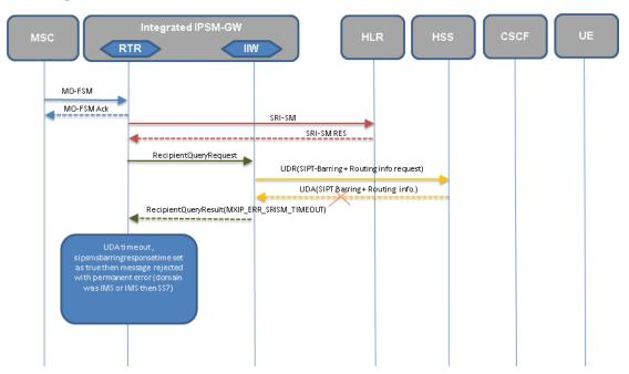
Figure 58: MO-SIPT message flow when the HSS query from the IIW times out
