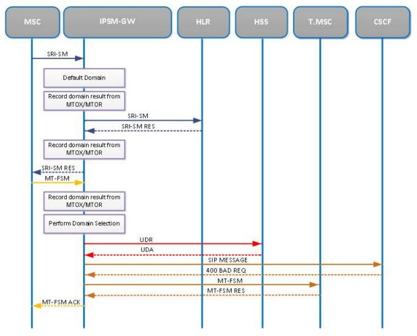
Figure 57: Domain Selection Mechanism Delivery for Home Routed Scenario
