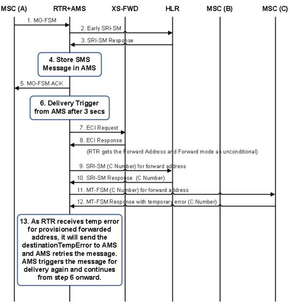
Figure 15: MO-Store-MT Scenario for unconditional XS-FWD service when rtrskipsrismforunconditional forwarding is true and Forwarded MT message Failure with temporary error
