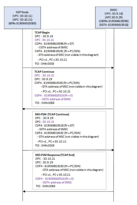
Figure 36: MO-FSM continue using TC-continue and closed using TC-End or Abort
