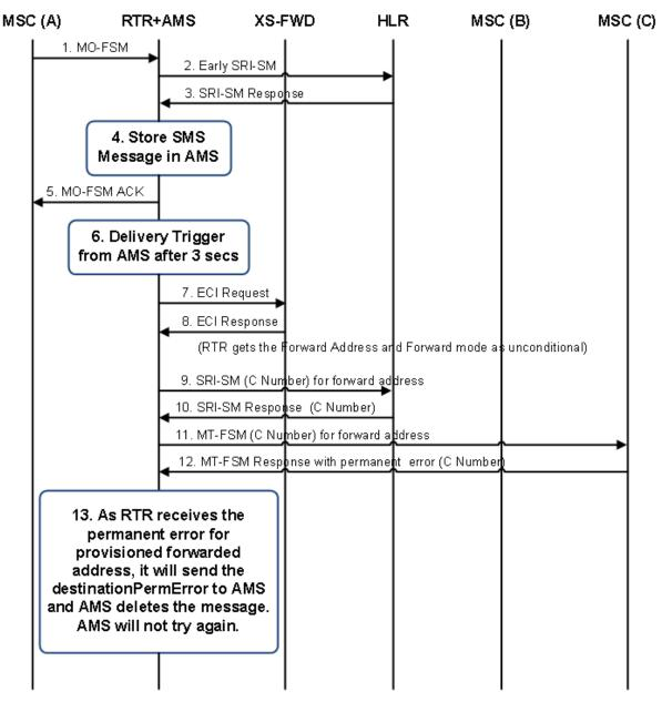
Figure 16: MO-Store-MT Scenario for unconditional XS-FWD service when rtrskipsrismforunconditional forwarding is true and Forwarded MT message Failure with permanent error
