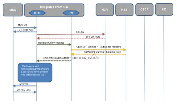
Figure 59: MO-SIPT message flow when the HSS query from the IIW times-out with fallback
