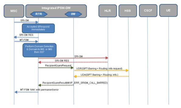
Figure 62: MT-SIPT scenario where SRISM performed After MT-FSM
