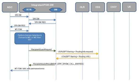
Figure 63: MT-SIPT scenario where SRISM performed before MT-FSM
